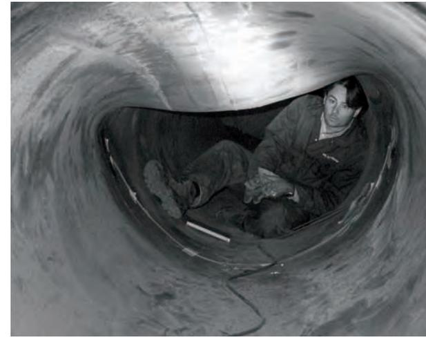
04 | View inside a (leak-proof) steel pipe after impact of an 18260 kg boulder dropped from a height of 18.85 m onto a gravel overburden of 1 m width: oval dent reducing the vertical diameter by approximately 30%
